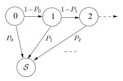
Fig. 6. State transition diagram for the number of slots required to select the best node after the first non-idle slot.
