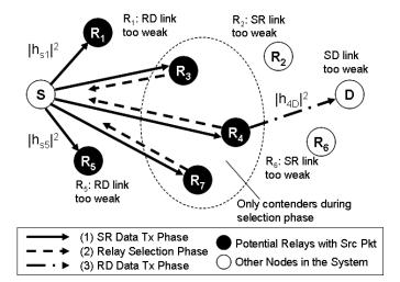
Fig. 1. A cooperative system consisting of a source (S), a destination (D), and n=7 relays.
