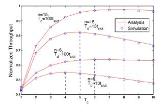
Fig. 3. Normalized throughput,  $\frac{\eta}{Wt_{\rm slot}}$ , as a function of number of slots in selection phase,  $T_c$ , for the non-adaptive system.
