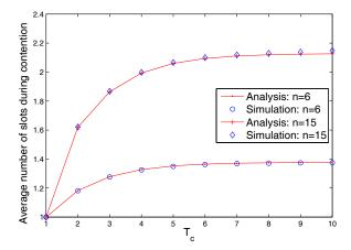
Fig. 4. Average number of slots required by the selection phase as a function of the maximum number of allowed contention slots for the adaptive selection duration system.
