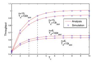
Fig. 5. Normalized throughput,  $\frac{\eta}{Wt_{\rm slot}}$ , as a function of the maximum number of allowed contention slots for the adaptive selection duration system.
