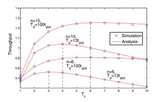
Fig. 6. Normalized throughput,  $\frac{\eta}{Wt_{\rm slot}}$ , as a function of the number of selection phase slots,  $T_c$ , when the RD data transmission duration is adapted (with  $T_{\rm max}=T_d$ ).
