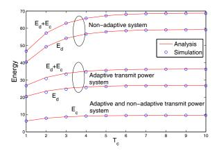
Fig. 7. Comparison of energy used by relays during the selection and RD data transmission phases for the non-adaptive and adaptive relay transmit power systems (with n=6 and  $T_d=13t_{\rm slot}$ ).
