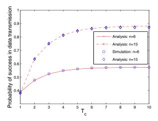
Fig. 2. Probability of successful selection,  $P_s(T_c)$ , as a function of number of slots in selection phase,  $T_c$ , for the non-adaptive system.
